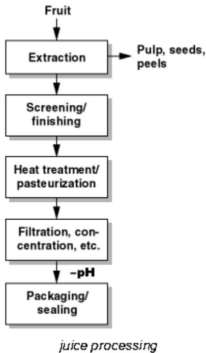
In juice processing, the contents of the fruit are extracted by squeezing or crushing. The pulp, seeds and peels are removed with screens in a finishing operation. The juice is then heat treated, filtered/concentrated as required by the particular product.
