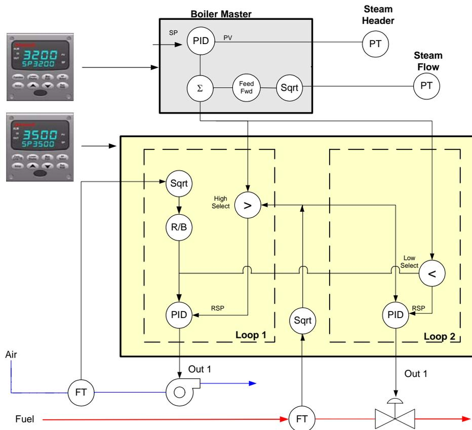
Figure 1 Lead-Lag, fuel/air ratio control plus demand control
